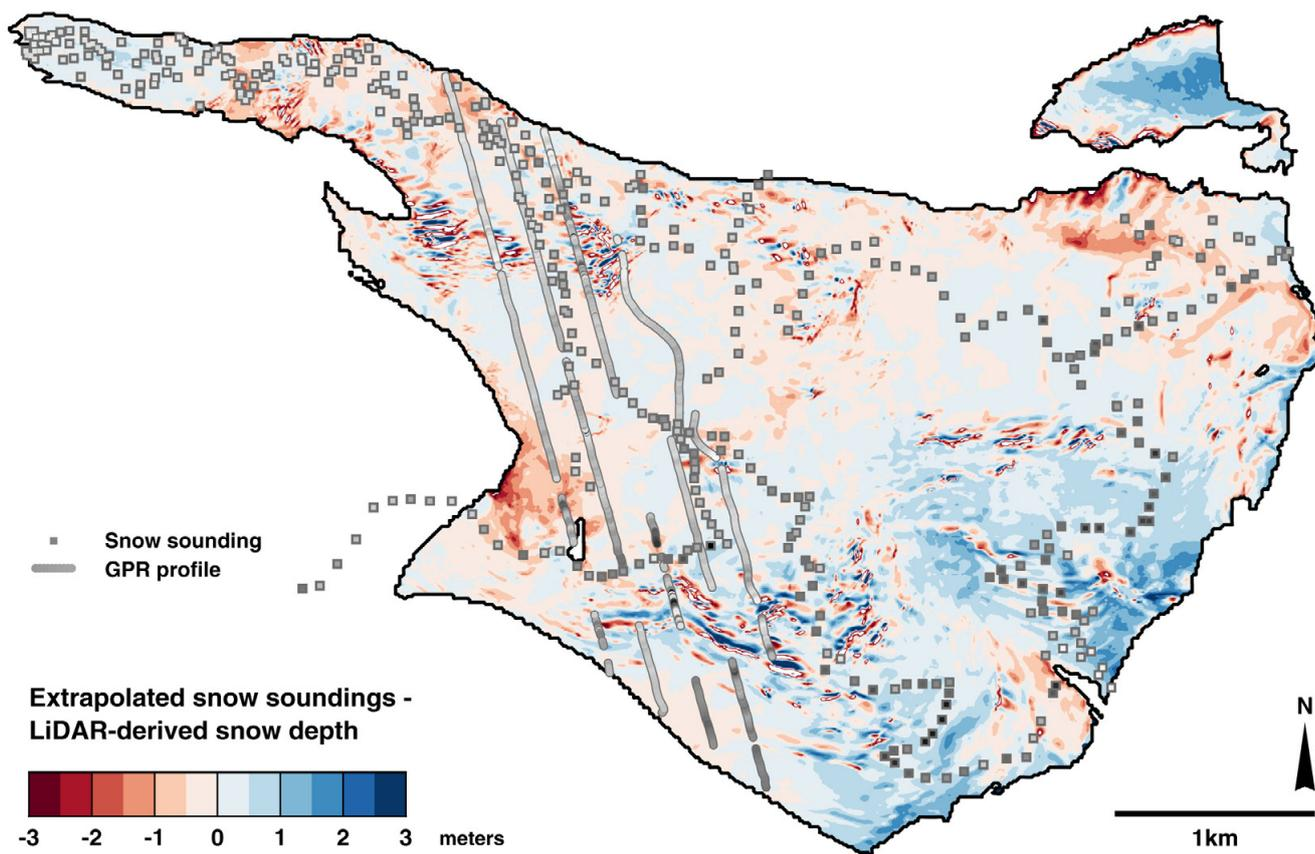
Figure 1. Snow soundings, GPR profile lines and difference between corrected LiDAR-derived snow depth and extrapolated snow soundings in April 2010 on Findelengletscher, Switzerland.
