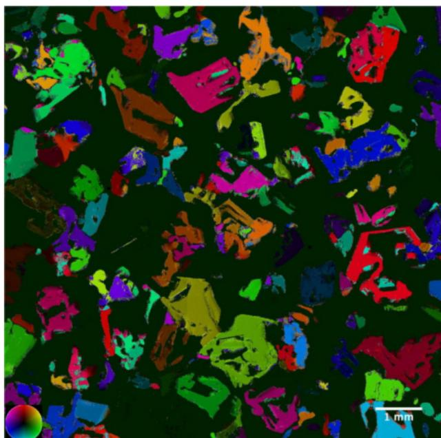
Figure 1. Depth hoar thin section analyzed with the Fabric analyzer G50. Each color corresponds to a different c-axis orientation of the snow crystals. C-axis orientation and color are related through a color wheel (bottom left).
