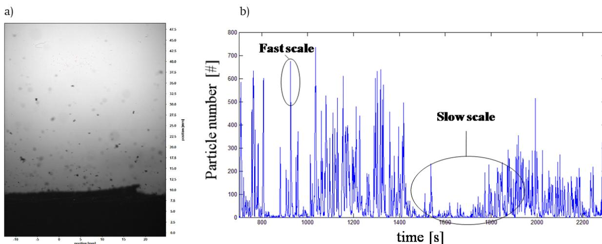
Figure 1. a) Shadowgraphic image (original size . b) Time series of particle number per image.
