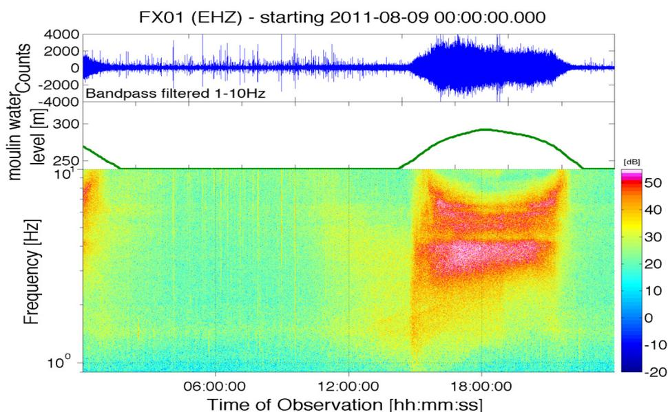
Figure 1. Spectrogram (bottom, unfiltered) and waveform (top, bandpass filtered 1-10 Hz) of the vertical component of the seismic signal during 24h of observations for a 1Hz LE-3D seismometer. The moulin water level (middle) correlates with the occurrence and shape of the seismic tremor.
