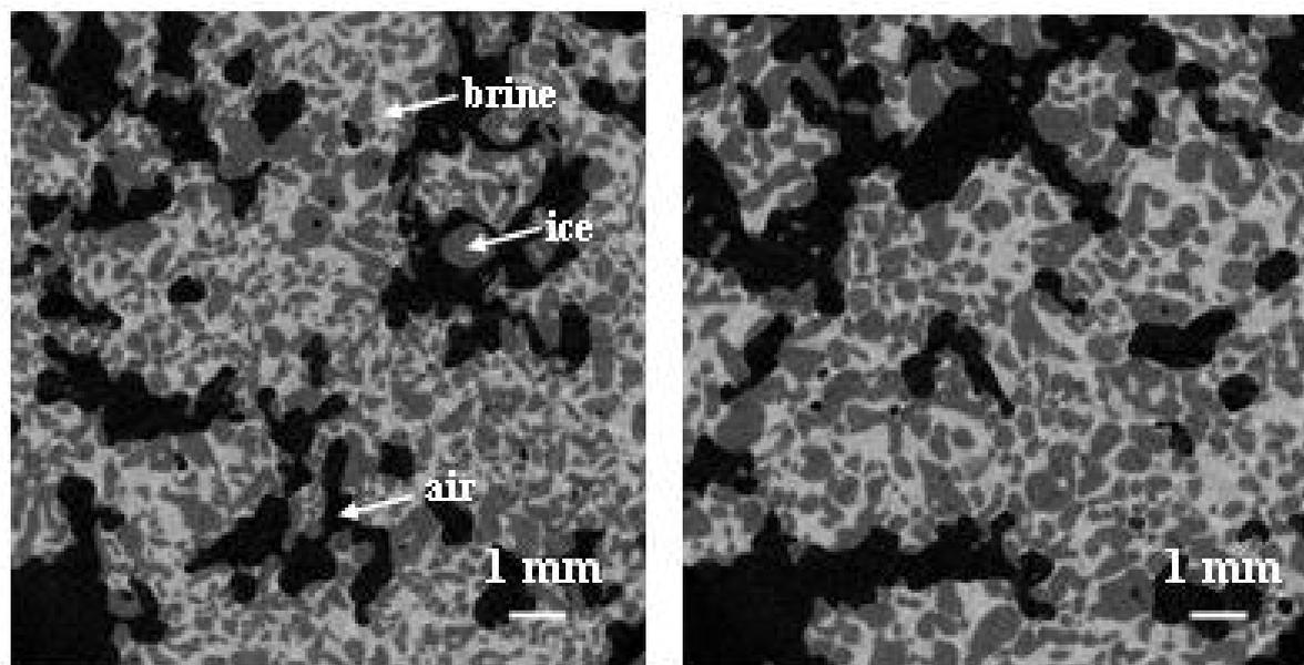
Figure 1) 2D micro-CT images of a salt-snow mixture with 45 w% NaCl measured at -18°C. *Left*: Sample immediately after adding and mixing with salt solution. *Right*: Same sample 21 days later.
