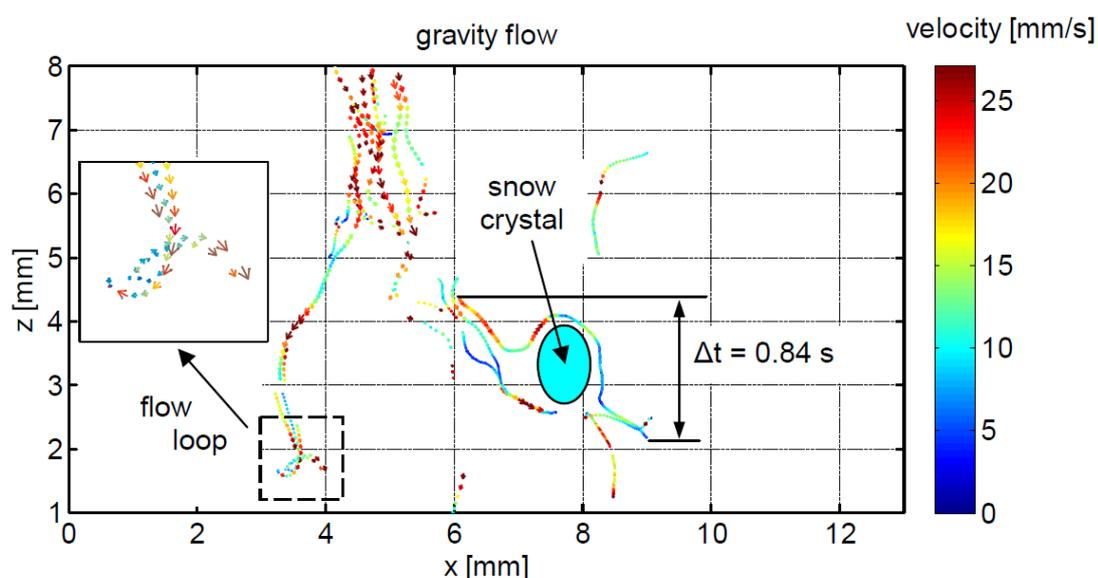
Figure 1. Particle trajectories for a gravity driven, saturated water flow in a wet snow sample. Colours of arrows indicate particle velocities.
