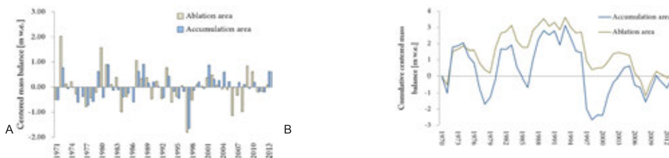
Figure 1. Centered (A) and cumulative centered (B) mass balance for a point location in the accumulation area and for one in the ablation area. From 1971 to 1994 and from 2012 to 2013 glaciological measurements and from 2001 to 2011 GPR data was used. Note that measurement gaps are filled in with the modeled mass balance at the point location.
