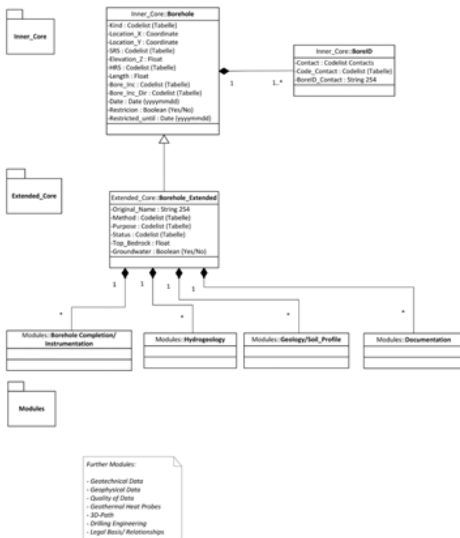
Figure 1. UML class diagram of the inner and extended core, as well different envisioned thematic modules. The Inner Core of the data model contains information which is always available without restriction. The Extended Core may contain information which is restricted.
